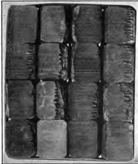
FIG. 89.—Brushes damaged due to pitting, glowing and under brush sparking occasioned by improper adjustment of the commutating field.
